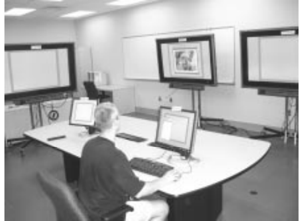
Figure 1: The interactive workspace used in our study. It consisted of two 20" LCD screens and three 61" plasma screens. Each screen had a label with a category name attached along the top that was used in the experimental task. A user viewed the current image in the application, relocated it to the screen with the appropriate label, redirected input to the local machine, typed an annotation, and redirected input back the screen with the application.
