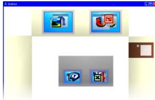
Figure 3. SEAPort also shows a spatial representation of the workspace. However, this interface uses fan-out views, zooming, and animation-based interactions to improve scalability and icons and portal views to improve awareness.
