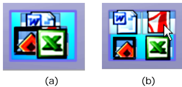
Figure 4. (a) A representation of a device with many applications, some of which are occluded. (b) The same device, but now shown in the fan-out view which eliminates the occlusion.
