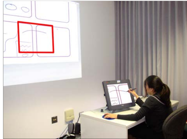
Figure 1: A user interacting with our focus+context system. She controls the frame of reference using her non-dominant hand while sketching with her dominant hand.
